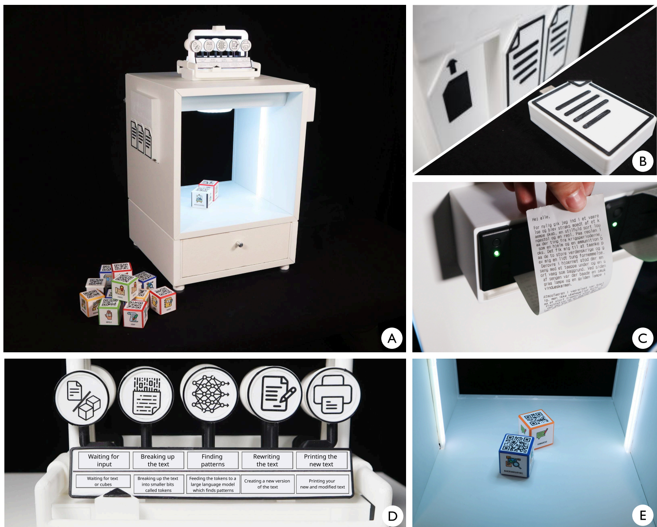
Figure 1: (A) The Prompt Machine. (B) Input module with three custom-made USB sockets and USB-textfiles for insertion. (C) Output module with two thermal printers. (D) Five-step tangible display. (E) Modification Canvas for inserting prompt cubes. From [7].
